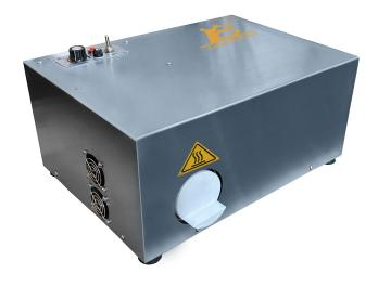
YB-R50 heat shrink machine, designed to encapsulate the end of a hose or tube assembly with a Clean Seal Capsule, Accepts Clean Seal Capsules from 0.87" I.D. (22mm) through 3" I.D. (80mm).
